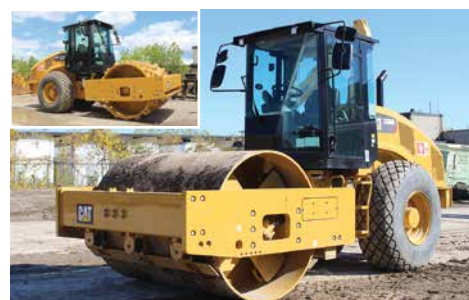
(2) NEW/UNUSED CAT CS66B 84" SMOOTH DRUM, A/C, CAB, PADSHELL KIT AVAILABLE.
